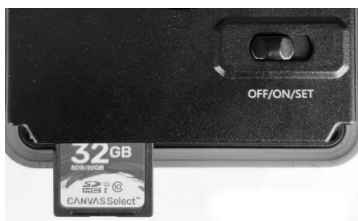
Figure 7: Inserting the SD Card
